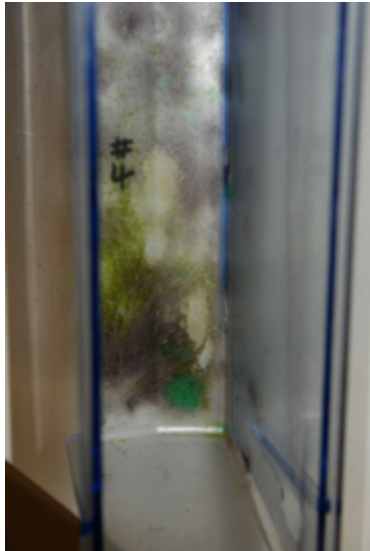
Figure. 7-1 Picture of a soiled tank with different algae types as well as biofilm noticeable
