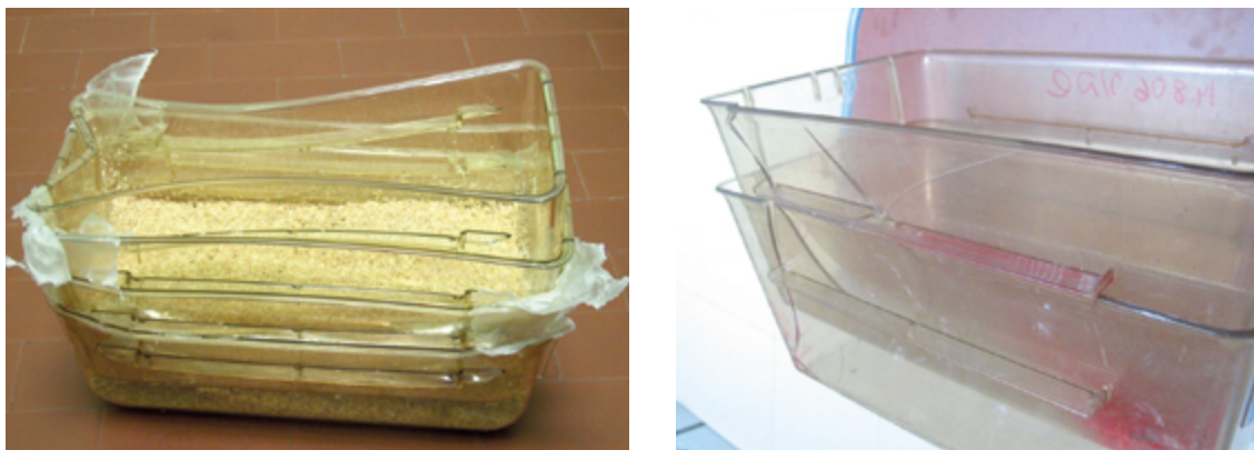
Figure 9-6 on the left deformation in cage bodies, on the right cracks in cage bodies
