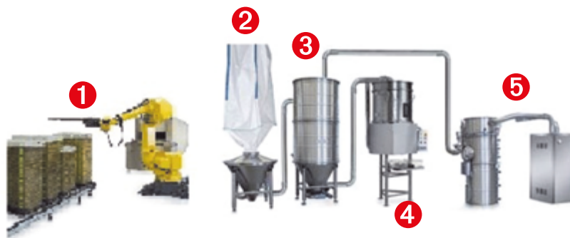
Fig. 4-17 Example for an fully automatic system: Filling of cages by robots or automatic machines ①, loading hopper e. g. for BIG-Bags ②, optional storage silo ③, dispenser with dust suction system ④ and vacuum generator and dust filter ⑤ for pneumatic conveyance
