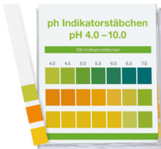
Figure 7-10 Example pH indicator sticks
