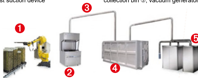
Figure 4-7 Example of a fully automatic system: automatic emptying with help of robots or machine ① into dumping hopper ②, with pneumatic waste conveyance with piping ③ into an external collection bin ④; vacuum generator and dust filter ⑤
